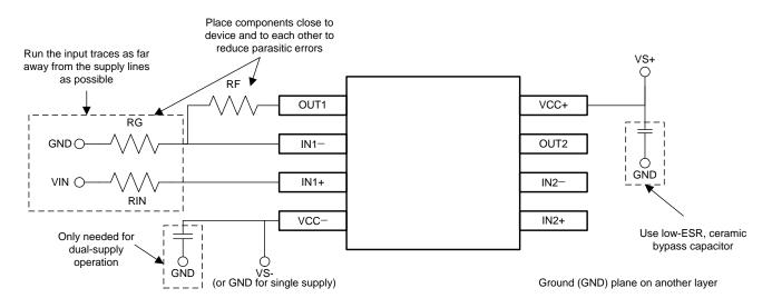
Figure 9. Operational Amplifier Board Layout for Noninverting Configuration
