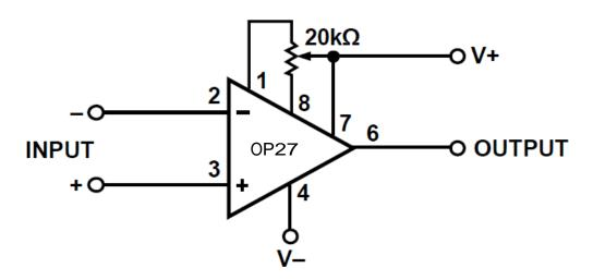
Figure 3.3 Optional Offset Nulling Circuit
