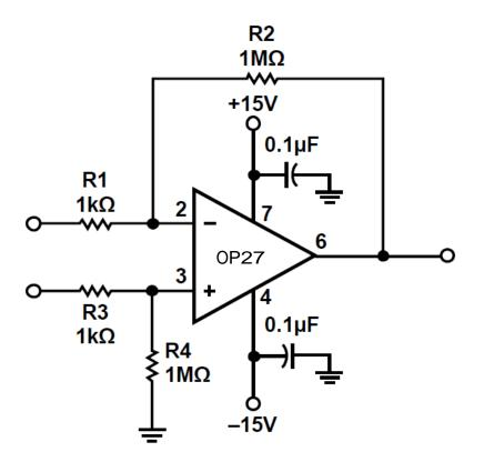
Figure 4.1 Precision High Gain Differential Circuit
