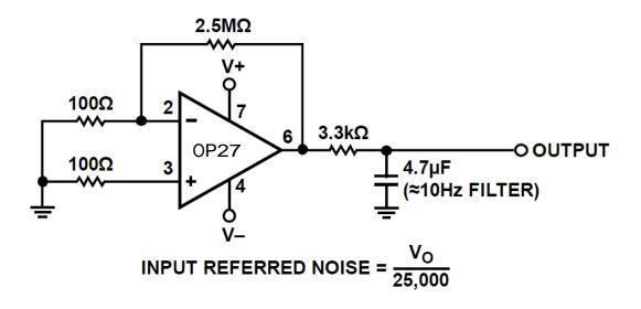
Figure 3.2 Typical Low Frequency Noise Test Circuit
