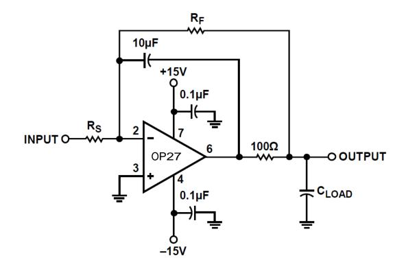
Figure 4.2 Isolating Large Capacitive Loads
