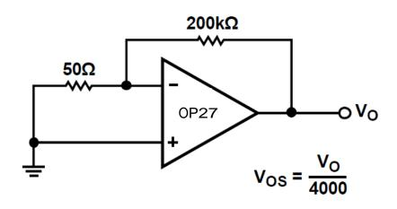
Figure 3.1 Typical Offset Voltage Test Circuit
