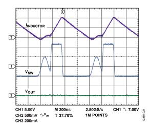
Figure 19. Discontinuous Conduction Mode Operation Showing Inductor Current ( $I_{INDUCTOR}$ ), Switch Node Voltage ( $V_{SW}$ ), and Output Ripple ( $V_{OUT}$ ),  $V_{IN} = 12 \text{ V}$ ,  $V_{OUT} = -5 \text{ V}$ ,  $I_{LOAD} = 100 \text{ mA}$ ,  $f_{SW} = 1.2 \text{ MHz}$ ,  $T_A = 25 ^{\circ}\text{C}$
