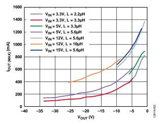
Figure 3. Maximum Output Current,  $f_{SW} = 1.2$  MHz,  $T_A = 25$  °C, Based on Target of 70%  $I_{LIM \, (MIN)}$
