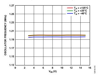
Figure 13. Oscillator Frequency vs. Input Voltage (V<sub>IN</sub>) for Various Temperatures, SYNC/FREQ Pin = Low
