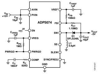
Figure 25. Typical +12 V Input to −5 V Output, 1.2 MHz Application
