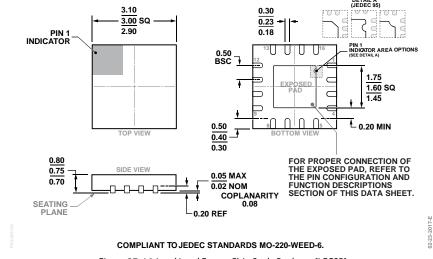
Figure 27. 16-Lead Lead Frame Chip Scale Package [LFCSP] 3 mm × 3 mm Body and 0.75 mm Package Height (CP-16-22) Dimensions shown in millimeters
