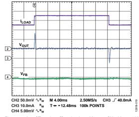
Figure 17. Load Transient Showing  $I_{LOAD}$ ,  $V_{OUT}$ , and  $V_{FB}$ ,  $V_{IN}=12~V$ ,  $V_{OUT}=-5~V$ ,  $I_{LOAD}=35~mA$  to 45~mA Step,  $f_{SW}=1.2~MHz$ ,  $T_A=25^{\circ}C$
