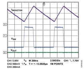
Figure 20. Continuous Conduction Mode Operation Showing Inductor Current ( $I_{INDUCTOR}$ ), Switch Node Voltage ( $V_{SW}$ ), and Output Ripple ( $V_{OUT}$ ),  $V_{IN} = 12 \text{ V}$ ,  $V_{OUT} = -5 \text{ V}$ ,  $I_{LOAD} = 250 \text{ mA}$ ,  $f_{SW} = 1.2 \text{ MHz}$ ,  $T_A = 25 ^{\circ}\text{C}$
