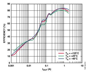
Figure 9. Efficiency vs. Current Load ( $I_{OUT}$ ) for Various Temperatures,  $V_{IN} = 5 V$ ,  $V_{OUT} = -15 V$ ,  $f_{SW} = 1.2 \text{ MHz}$
