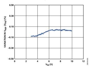
Figure 10. Line Regulation,  $V_{OUT} = -5 V$ ,  $f_{SW} = 1.2 MHz$ , 15 mA Load,  $T_A = 25 ^{\circ}C$  (Skip Mode Not Shown)
