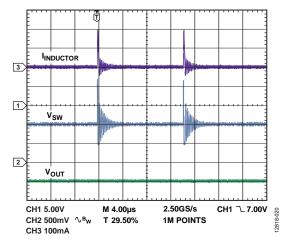
Figure 18. Skip Mode Operation Showing Inductor Current ( $I_{INDUCTOR}$ ), Switch Node Voltage ( $V_{SW}$ ), and Output Ripple ( $V_{OUT}$ ),  $V_{IN} = 12$  V,  $V_{OUT} = -5$  V,  $I_{LOAD} = 1$  mA,  $f_{SW} = 1.2$  MHz,  $T_A = 25$ °C
