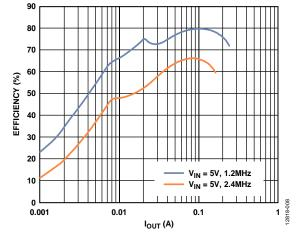
Figure 8. Efficiency vs. Current Load ( $I_{OUT}$ ),  $V_{IN} = 5$  V,  $V_{OUT} = -30$  V,  $T_A = 25$ °C
