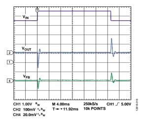
Figure 16. Line Transient Showing  $V_{IN,V}$   $V_{OUT}$ , and  $V_{FB}$ ,  $V_{IN}$  = 4.5 V to 5.5 V Step,  $V_{OUT}$  = -5 V,  $R_{LOAD}$  =  $300~\Omega$ ,  $f_{SW}$  = 1.2 MHz,  $T_A$  = 25°C
