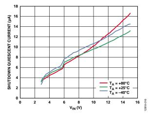
Figure 14. Shutdown Quiescent Current (I<sub>SHDN</sub>) vs. Input Voltage (V<sub>IN</sub>) for Various Temperatures, EN Pin Below Shutdown Threshold
