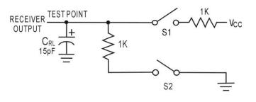
Figure 1. Driver DC Test Load
