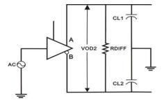
Figure3. Driver Timing Test Load
