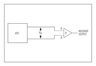
Figure 9. Receiver Propagation Delay Test Circuit
