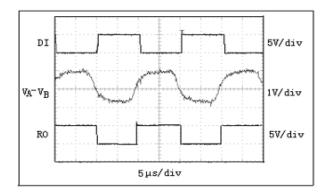
Figure 13. GM75176E System Differentia Voltage at 50kHz Driving 4000ft of Cable
