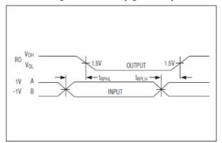
Figure 7. Receiver Propagation Delays
