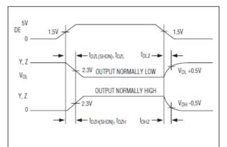
Figure6. Driver Enable and Disable Times
