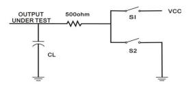
Figure 4. Driver Enable/Disable Timing Test Load
