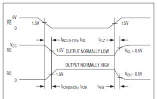
Figure8. Receiver Enable and Disable Times
