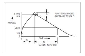
Figure 10b. Human Body Current Waveform
