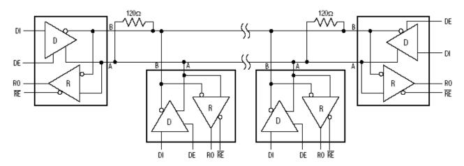
Figure 14. GM75176E Pin Configuration and Typical Half-Duplex Operating Circuit
