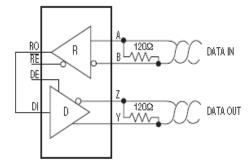
Figure 12. Line Repeater for GM75176E
