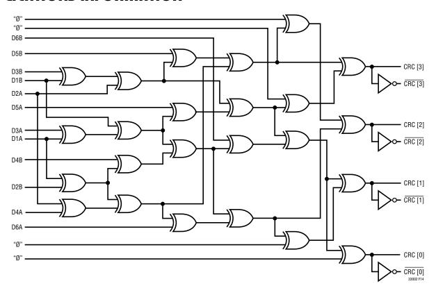
Figure 14. Combinational Logic Circuit Implementation of the CRC Calculator
