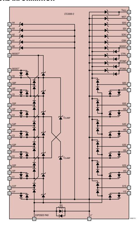
Figure 12. Internal Protection Diodes
