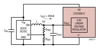
Figure 11. Adding External Buck DC/DC for >40mA V<sub>REG</sub> Drive
