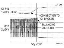
Protection for Broken Connection to Secondary Stack While Discharging
