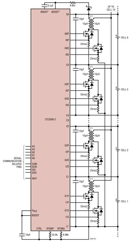
Figure 3. LTC3300-2 6-Cell Active Balancer Module Showing Power Connections for the Multi-Transformer Application (CTRL =  $V^-$ )
