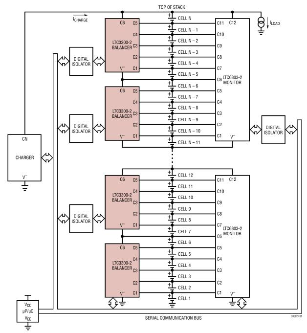
Figure 1. LTC3300-2/LTC6803-2 Typical Battery Management System (BMS)
