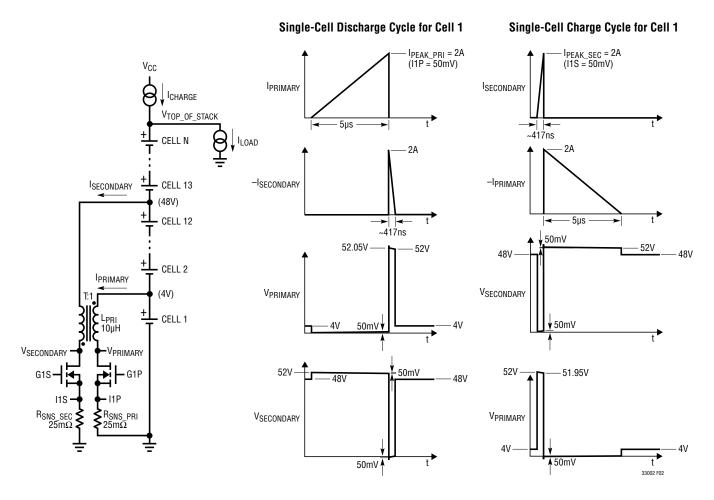
Figure 2. Synchronous Flyback Balancing Example with T = 1, S = 12
