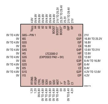
Figure 15. Typical Pin Voltages for Six 4.2V Cells
