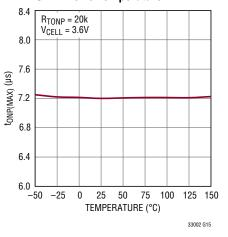
Secondary Winding Switch Maximum On-Time vs Temperature
