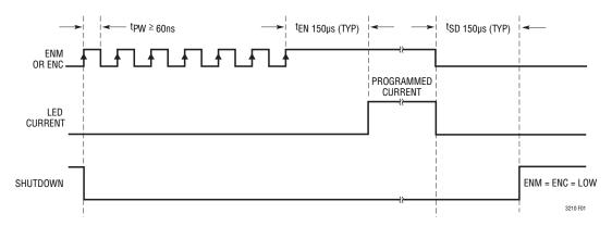
Figure 1. Current Programming and Shutdown Timing Diagram
