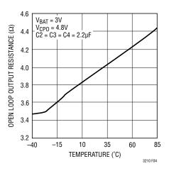
Figure 4. Typical 2x R<sub>OL</sub> vs Temperature
