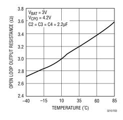
Figure 3. Typical 1.5x R<sub>OL</sub> vs Temperature
