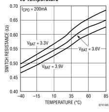
1.5x Mode Charge Pump Open-Loop Output Resistance vs Temperature  $(1.5V_{BAT} - V_{CPO})/I_{CPO}$
