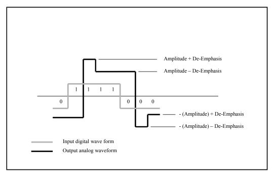
Figure 5-1 Driver Output Waveform
