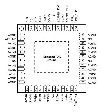
Exposed pad is system GND, must be soldered to PCB ground plane
