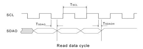
Figure 11 EEPROM Command Cycle Timing Diagram
