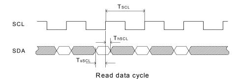
Figure 9 EEPROM Read Cycle Timing Diagram
