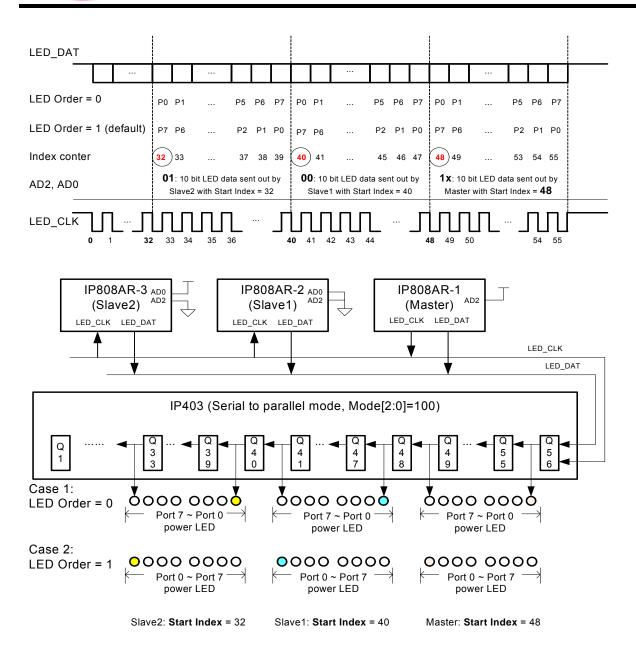
Figure 6 LED behavior and system diagram of multiple IP808AR application
