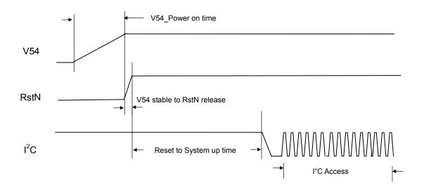
Figure 8 Power on Sequence and Reset Timing Diagram
