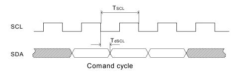
Figure 10 EEPROM Command Cycle Timing Diagram
