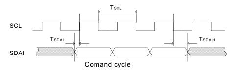
Figure 12 I<sup>2</sup>C Command Cycle Timing Diagram
