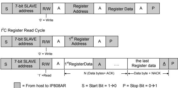
Figure 4 I<sup>2</sup>C bus read/write cycles diagram
