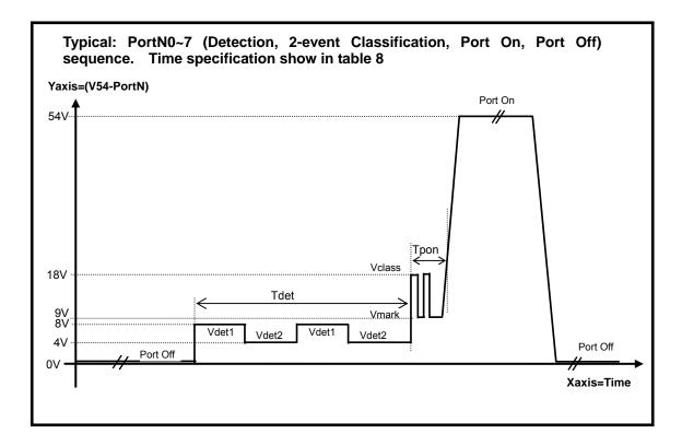
Figure 7 Typical Power up Sequence
