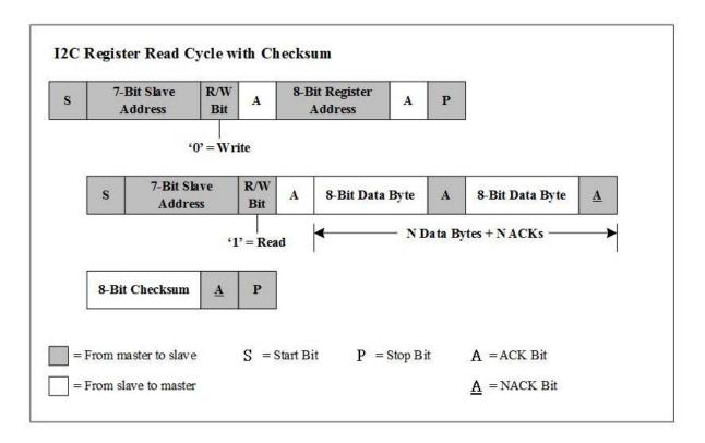
The 8-bit checksum for I2C read cycle is calculated as the following:
