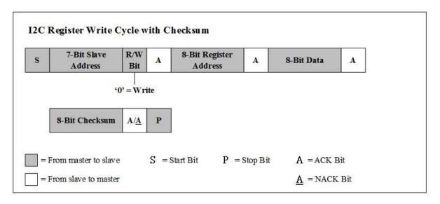
The 8-bit checksum for I2C write cycle is calculated as the following:
