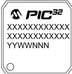
100-Lead TQFP (12x12x1 mm)
