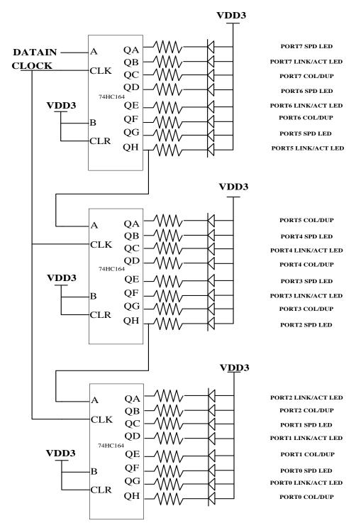
**Exteranl TTL for 3 Bit Serial Stream LED Mode**
