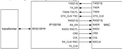
MII is active if pin 36 RGMII\_N/GMII is pulled high and IP1001 islinked at 100M, or 10M.
