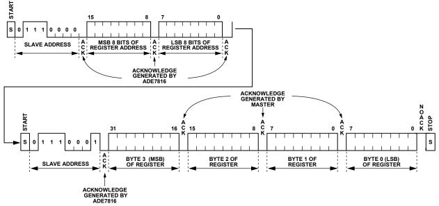
Figure 44. I<sup>2</sup>C Read Operation of a 32-Bit Register Rev. B | Page 34 of 48
