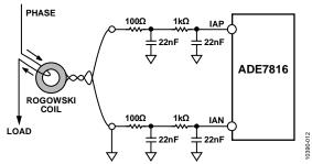
Figure 27. Rogowski Coil Input Connections
