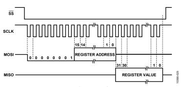
Figure 45. SPI Read Operation of a 32-Bit Register
