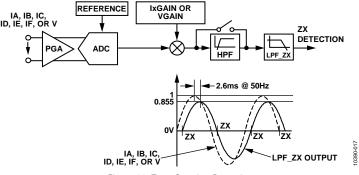
Figure 33. Zero-Crossing Detection
