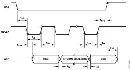
Figure 4. HSDC Interface Timing
