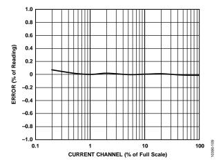
Figure 15. I<sub>RMS</sub> Error as a Percentage of Reading (Gain = 1, Temperature = 25°C, Power Factor = 1) with Internal Reference, Integrator Off
