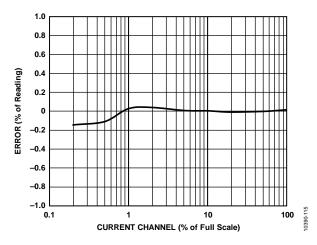
Figure 21. I<sub>RMS</sub> Error as a Percentage of Reading (Gain = 16, Temperature = 25°C, Power Factor = 1) with Internal Reference, Integrator On
