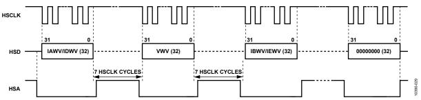
Figure 49. HSDC Communication for HSIZE = 0, HGAP = 1, HXFER[1:0] = 01, and HSAPOL = 0
