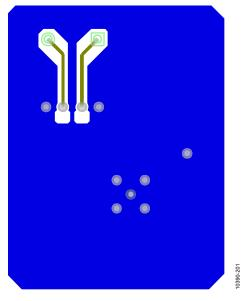
Figure 40. Bottom Layer Printed Circuit Board
