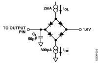
Figure 5. Load Circuit for All Timing Specifications
