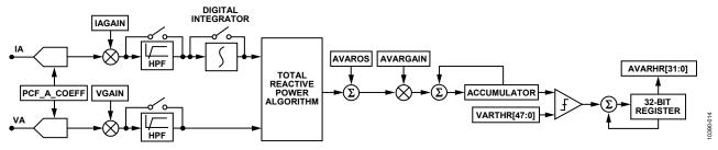
Figure 29. Reactive Energy Signal Path
