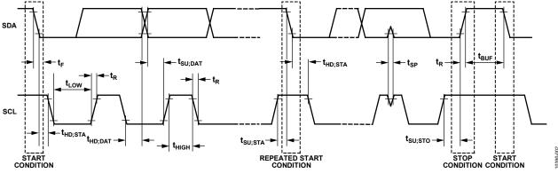
Figure 2. I<sup>2</sup>C-Compatible Interface Timing
