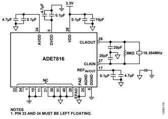
Figure 38. Crystal and Capacitors Connection
