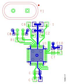
Figure 39. Recommended Decoupling Capacitors Layout
