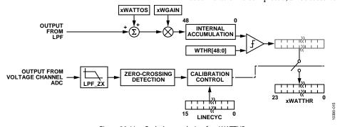
Figure 30. Line Cycle Accumulation for xWATTHR
