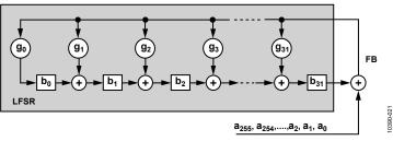
Figure 37. LFSR Generator Used in Checksum Register Calculation
