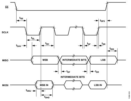
Figure 3. SPI Interface Timing
