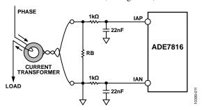
Figure 26. Current Transformer Input Connections
