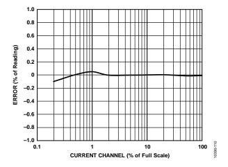
Figure 16. V<sub>RMS</sub> Error as a Percentage of Reading (Gain = 1, Temperature = 25°C, Power Factor = 1) with Internal Reference, Integrator Off
