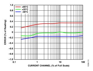
Figure 19. Reactive Energy Error as a Percentage of Reading (Gain = 16, Power Factor = 0) over Temperature with Internal Reference, Integrator On
