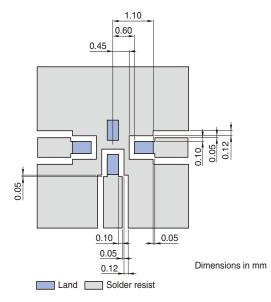
Line width should be designed to match  $50\Omega$  characteristic impedance, depending on PCB material and thickness.
