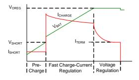
(b) Charge Curve, I<sub>IN LIMIT</sub> Limits I<sub>CHARGE</sub>
