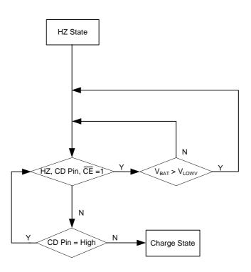
Figure 5. HZ State Flow Chart
