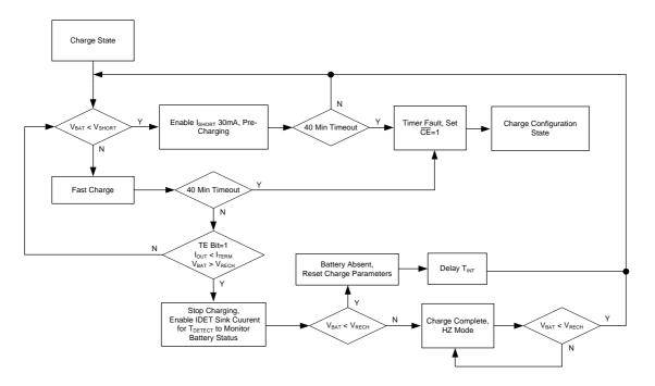
Figure 7. Operational Flow Chart in Charge Mode
