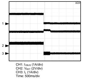
DPM,  $V_{SP}$ =4.533V,  $V_{OREG}$ =4.2V,  $V_{BAT}$ =3.8,  $I_{IN\_LIMIT}$ =NO Limit, TE=1
