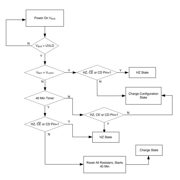
Figure 4. Charger VBUS POR Flow Chart
