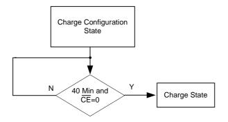
Figure 6. Charge Configuration Flow Chart
