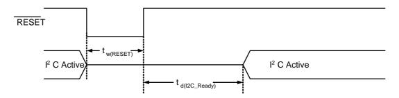
Figure 3. Reset Timing
