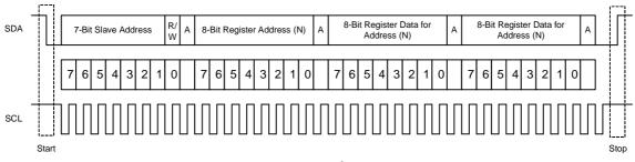
Figure 10. Typical I<sup>2</sup>C sequence
