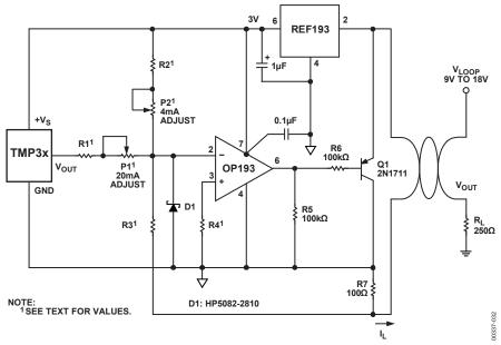
Figure 33. Temperature to 4–20 mA Loop Transmitter
