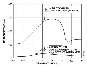
Figure 15. V<sub>OUT</sub> Response Time for SHUTDOWN Pin vs. Temperature
