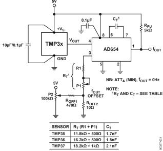
Figure 34. Temperature-to-Frequency Converter
