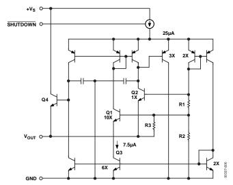
Figure 22. Temperature Sensor Simplified Equivalent Circuit
