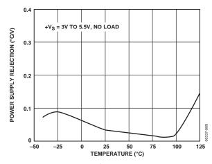
Figure 8. Power Supply Rejection vs. Temperature
