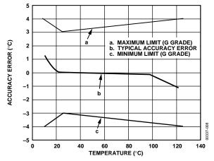
Figure 7. Accuracy Error vs. Temperature
