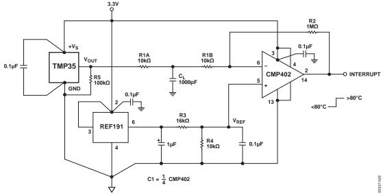
Figure 30. Microprocessor Overtemperature Interrupt Generator
