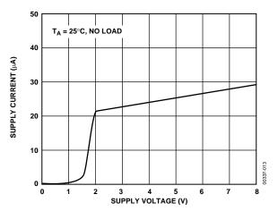
Figure 12. Supply Current vs. Supply Voltage
