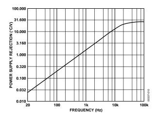
Figure 9. Power Supply Rejection vs. Frequency
