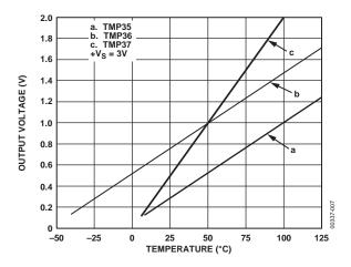
Figure 6. Output Voltage vs. Temperature
