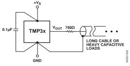
Figure 35. Driving Long Cables or Heavy Capacitive Loads
