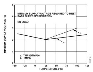
Figure 10. Minimum Supply Voltage vs. Temperature
