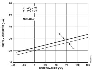
Figure 11. Supply Current vs. Temperature
