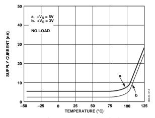
Figure 13. Supply Current vs. Temperature (Shutdown = 0 V)
