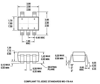
Figure 37. 5-Lead Small Outline Transistor Package [SOT-23] (RJ-5) Dimensions shown in millimeters
