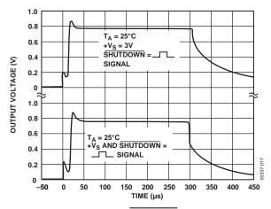
Figure 16. Vout Response Time to SHUTDOWN Pin and +Vs Pin vs. Time
