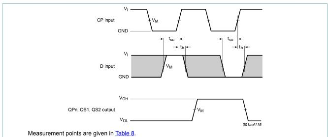
$V_{OL}$  and  $V_{OH}$  are typical voltage output levels that occur with the output load.
