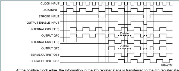
At the positive clock edge, the information in the 7th register stage is transferred to the 8th register stage and the QSn outputs.
