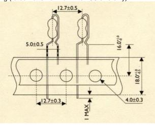
AV Type Forming for Taping (rated watts from 1/4W to 2SS size only)
