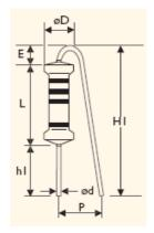
**STYLE DIMENSIONS** UNIT: mm Ψd Normal Miniature L ψd h1 H1 max E max HHV-50 HHV1SS  $9.0 \pm 0.5$ 3.3± 0.3 0.55± 0.05  $6.0 \pm 1$  $5.0 \pm 1$ 18.5 3.5 HHV1WS HHV2SS  $11.5 \pm 1.0$  $4.5 \pm 0.5$  $0.8 \pm 0.05$  $6.0 \pm 1$  $5.0 \pm 1$ 20 3.5 HHV2WS HHV3SS  $15.5 \pm 1.0$  $5.0 \pm 0.5$  $0.8 \pm 0.05$  $8.0 \pm 1$  $5.0 \pm 1$ 25 3.5
