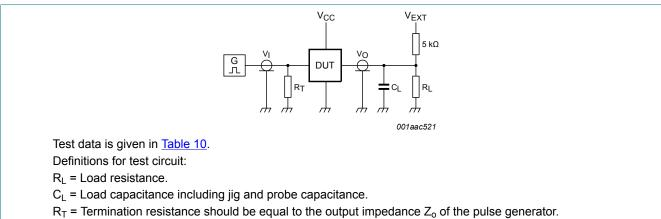
V<sub>EXT</sub> = External voltage for measuring switching times.
