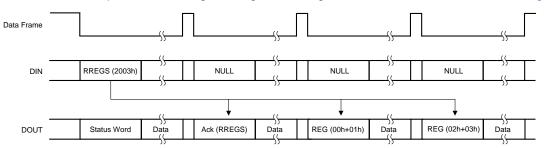
Figure 76. RREGS Command Status Response (Multiple Register Read)
