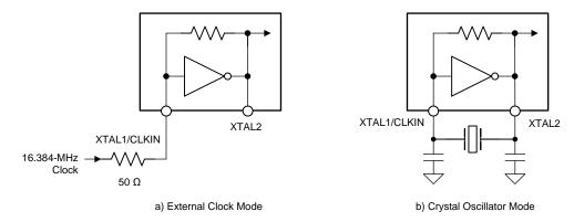
Figure 36. Clock Mode Configurations
