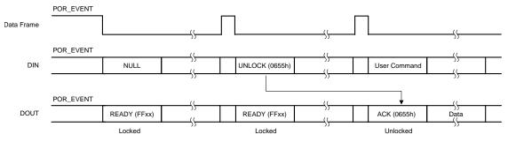
Figure 74. UNLOCK from a POR Command Status Response
