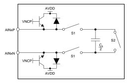
Figure 38. Equivalent Analog Input Circuitry
