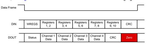
Figure 57. CRC Using the WREGS Command
