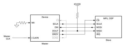
Figure 63. Synchronous Master Mode Device Connections
