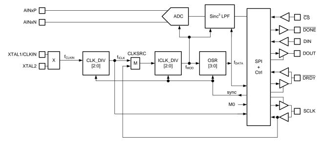
Figure 35. ADC Clock Generation
