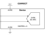
Charge pump disabled with unipolar analog supply, AVDD > 3.6 V.
