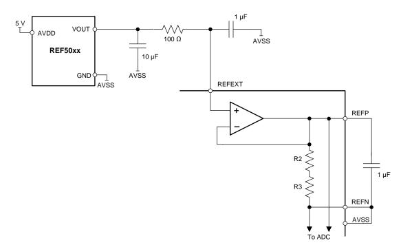
NOTE:  $R2 = 62.3 \text{ k}\Omega$ ,  $R3 = 97.5 \text{ k}\Omega$ .
