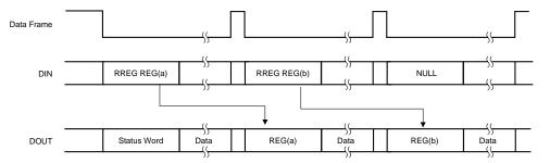
Figure 75. RREGS Command Status Response (Single Register Read)
