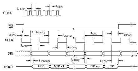
NOTE: SPI settings are CPOL = 0 and CPHA = 1.  $\overline{CS}$  can be tied directly to  $\overline{DRDY}$ .
