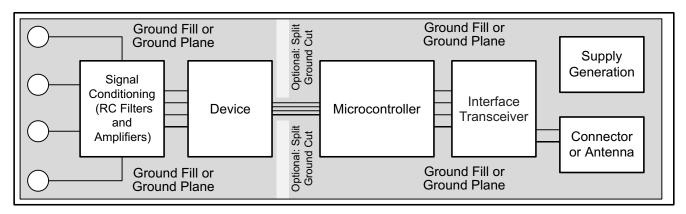
Figure 110. System Component Placement
