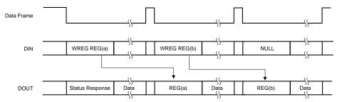
Figure 77. WREG Command Status Response (Single Register Write)
