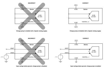
Figure 105. Correct and Incorrect Circuit Connections, Continued
