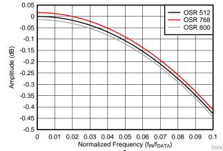
Figure 50. Non-Binary OSR Sinc<sup>3</sup> Filter Frequency Response
