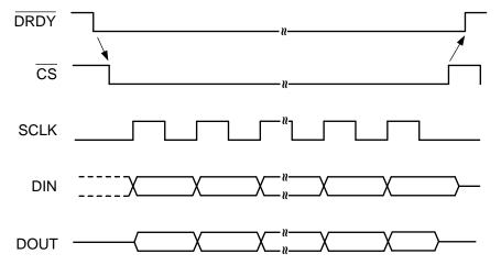
Figure 62. DRDY Behavior with Data Retrieval in Asynchronous Interrupt Mode
