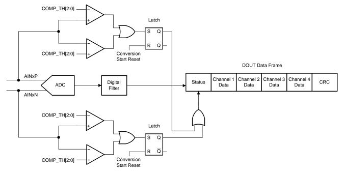
Figure 42. ADC Out-of-Range Detection Monitor
