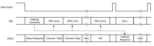
Figure 78. WREGS Command Status Response (Multiple Register Write)
