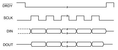
Figure 64. Data Retrieval in Synchronous Master Mode
