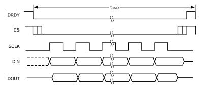
Figure 66. Data Retrieval in Synchronous Slave Mode
