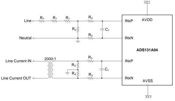
Figure 102. Typical Power Metering Connections
