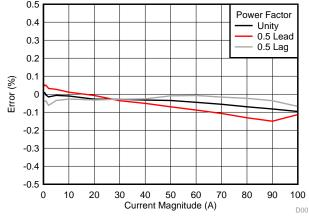
Figure 103. Active Power Measurement Error
