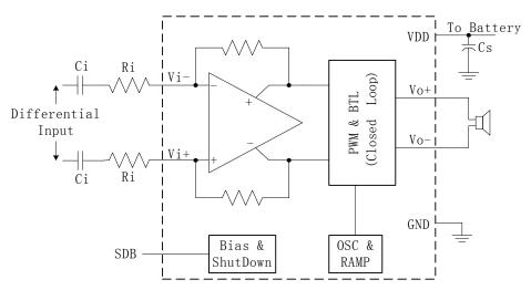
Figure 3. BL6306 Application Schematic With Differential Input and Input Capacitors
