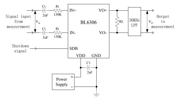
Figure 5. BL6306 test set up circuit
