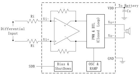
Figure 2. BL6306 Application Schematic With Differential Input
