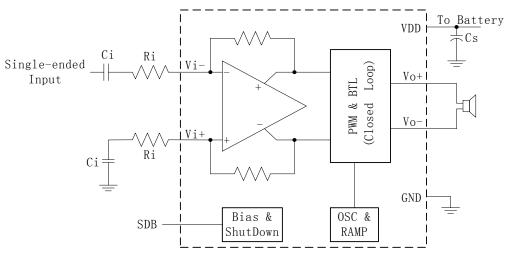
Figure 4. BL6306 Application Schematic With Single-Ended Input
