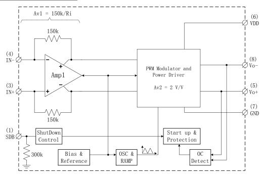
**Notes:** Total Voltage Gain =  $Av1 \times Av2 = 2 \times \frac{150k}{R_1}$
