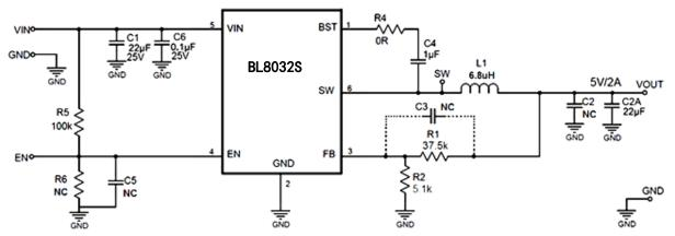
Figure1. 12V VIN, 5V/2A
