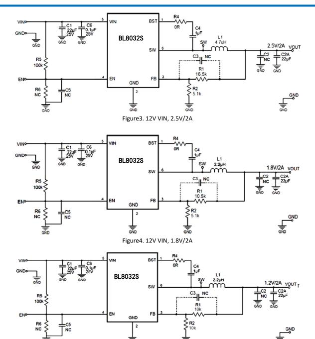
Figure 5. 12V VIN, 1.2V/2A
