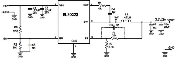
Figure 2. 12V VIN, 3.3V/2A
