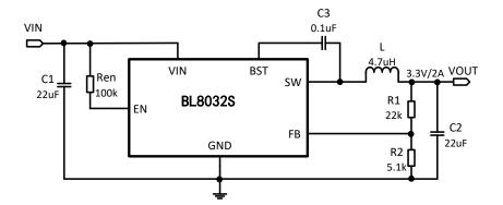
**Note:** 1) C1 and C2 recommended using 22uF ceramic capacitors. If the electrolytic capacitor is used, it is recommended that the ceramic capacitor in parallel with a capacitance value of 0.1uF or more.
