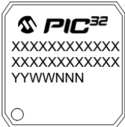
100-Lead TQFP (14x14x1 mm)
