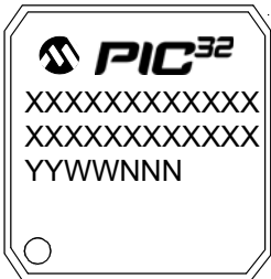
100-Lead TQFP (12x12x1 mm)
