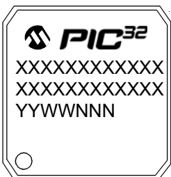
100-Lead TQFP (14x14x1 mm)
