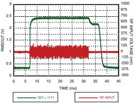
Figure 8.Residual Ripple for 1900 MHz WCDMA4C @ SCI=1111
