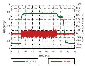
Figure 10.Residual Ripple for 1900 MHz LTE @ SCI=1111
