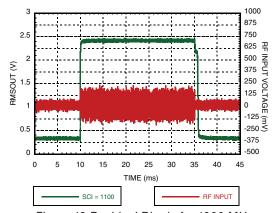
Figure 12.Residual Ripple for 1900 MHz GSM6C @ SCI=1100
