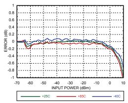
Figure 17.Reading Error for LTE wrt CW Response
