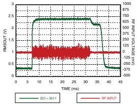
Figure 13.Residual Ripple for 1900 MHz LTE @ SCI=1111
