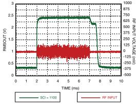
Figure 7.Residual Ripple for 1900 MHz WCDMA4C @ SCI=1100
