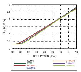
RMSOUT vs. Pin w/ CW & LTE 20MHz @ 1900 MHz & +25 °C [1]
