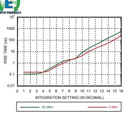
Figure 4.Rise Time<sup>[2]</sup> vs. SCI Setting over Input Power
