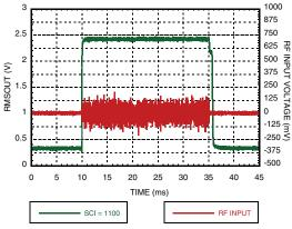
Figure 9.Residual Ripple for 1900 MHz LTE @ SCI=1100
