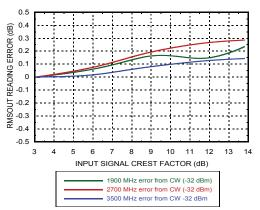
Figure 18.RMSOUT Error vs. Crest Factor over Frequency
