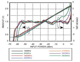
Figure 1.RMSOUT & Error vs. Pin
