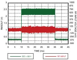
Figure 11.Residual Ripple for 1900 MHz GSM6C @ SCI=0011
