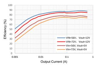
Figure 3. Efficiency vs Load Current
