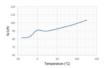
Figure 7. Iq vs Temperature
