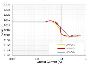
Figure 4. Load Regulation (Vout=12V)
