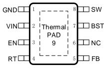
Figure 1. 8-Lead Plastic E-SOP
