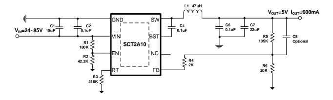
Figure 11. SCT2A10 Design Example, 5V Output with Programmable UVLO
