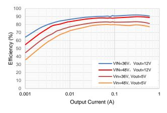
Figure 2. Efficiency vs Load Current
