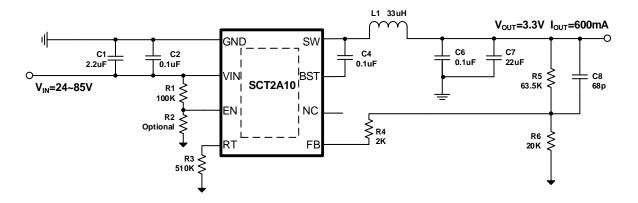
Figure 12. VOUT=3.3V, IOUT=0.6A Application Circuit
