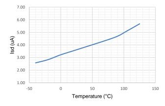
Figure 6. Shut-down Current vs Temperature
