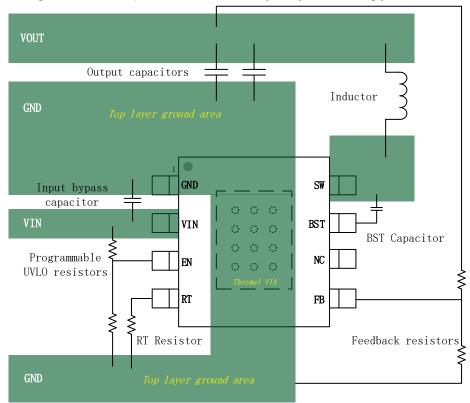
Figure 26. PCB Layout Example
