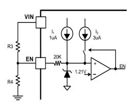
Figure 9. System UVLO by enable divide
