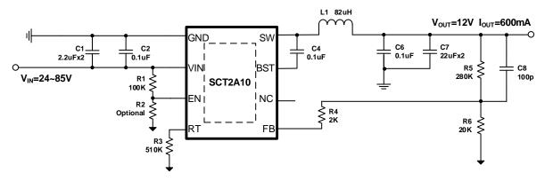
Figure 14. VOUT=12V, IOUT=0.6A Application Circuit
