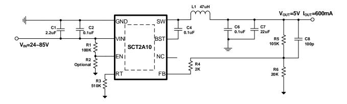
Figure 13. VOUT=5V, IOUT=0.6A Application Circuit
