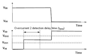
Figure 4. Overcurrent delay time
