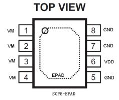
Figure 2. PIN Configuration
