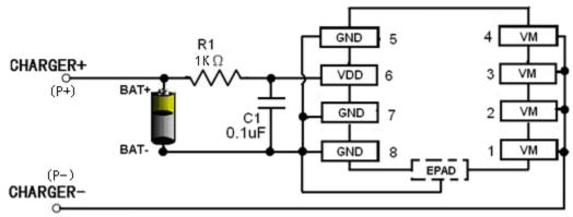
Figure 1. Typical Application Circuit
