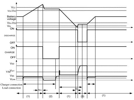
Figure 5-1 Overcharge and Overdischarge Voltage Detection
