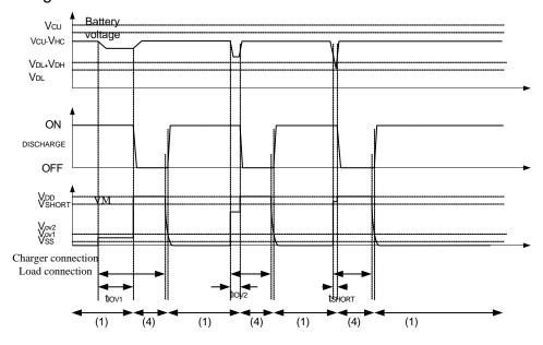
**Figure5-2 Overdischarge Current Detection**
