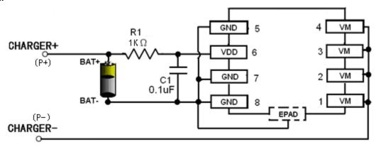
Fig 6 XB8889A in a Typical Battery Protection Circuit
