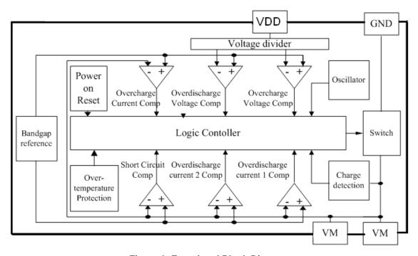
Figure 3. Functional Block Diagram
