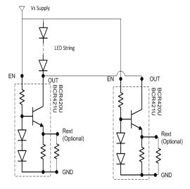
Figure 2 Application Circuit for Increasing LED Current
