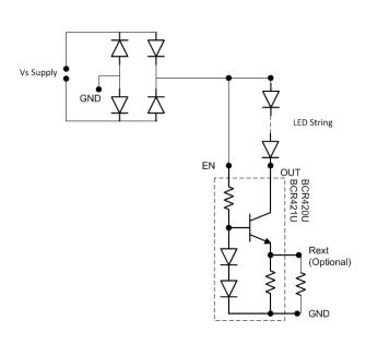
Figure 6 Application Circuit for LED Driver with Assured Operation Regardless Of Polarity
