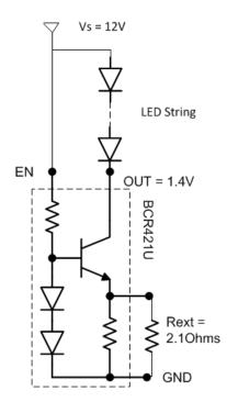
Figure 7 Example for 350mA Operation
