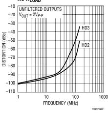
Distortion (Unfiltered) vs Frequency, Single-Ended Input,  $R_{LOAD} = 400\Omega$
