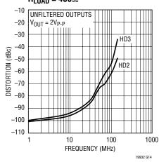
Distortion (Unfiltered) vs Frequency, Differential Input,  $R_{LOAD}$  =  $100\Omega$
