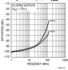
Distortion (Filtered) vs Frequency Single-Ended Input,  $R_{LOAD} = 400\Omega$
