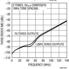
Third Order Intermodulation Distortion vs Frequency Differential Input,  $R_{LOAD} = 400\Omega$
