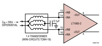
Figure 4. Input Termination for Differential 50  $\!\Omega$  Input Impedance with 6dB Additional Gain
