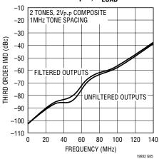
Third Order Intermodulation Distortion vs Frequency Differential Input,  $R_{LOAD} = 100\Omega$
