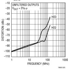
Distortion (Unfiltered) vs Frequency, Single-Ended Input,  $R_{LOAD} = 100 \Omega$
