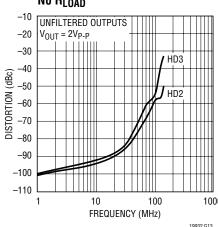
Distortion (Unfiltered) vs Frequency, Differential Input,  $R_{LOAD} = 400\Omega$
