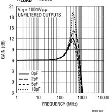
Frequency Response  $R_{LOAD} = 100\Omega$
