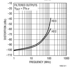
Distortion (Filtered) vs Frequency Differential Input,  $R_{LOAD}$  = 100 $\Omega$
