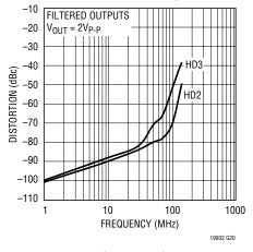
Distortion (Filtered) vs Frequency Single-Ended Input,  $R_{LOAD}$  = 100  $\!\Omega$
