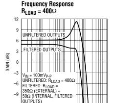
Frequency Response vs  $C_{LOAD}$ ,  $R_{LOAD} = 400\Omega$
