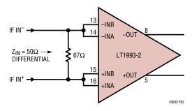
Figure 3. Alternate Input Termination for Differential  $\mathbf{50}\Omega$  Input Impedance
