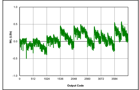
FIGURE 45-94: ADC 12-bit Mode, Single-Ended INL, V_{DD} = 3.0V , V_{REF} = 3.0V , T_{AD} = 1 \mu S , CP ON, 25°C.
