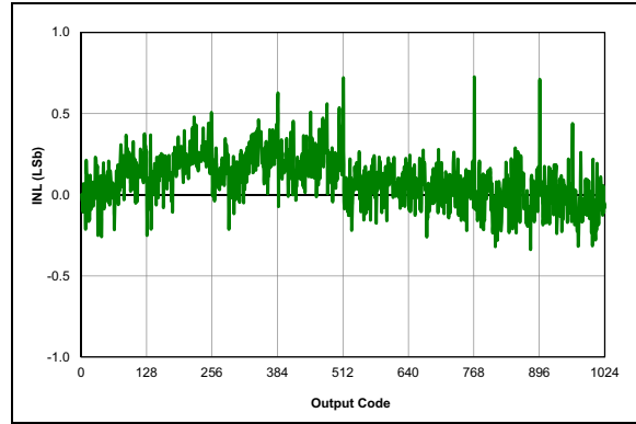
FIGURE 38-80: ADC 10-bit Mode, Single-Ended INL, V_{DD} = 3.0V , T_{AD} = 1\ \mu\text{S} , 25^\circ\text{C} .
