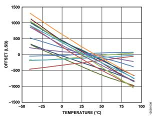
Figure 8. Y-Axis Offset vs. Temperature (N = 16)
