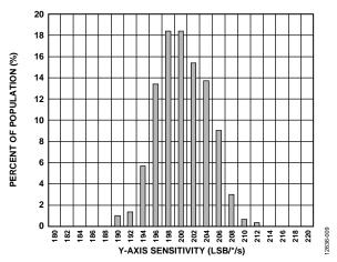
Figure 9. Y-Axis Sensitivity at 25°C
