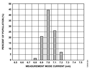
Figure 22. Measurement Mode Current Consumption
