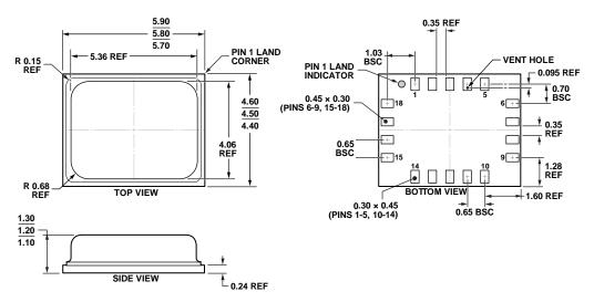
Figure 36. 18-Terminal Chip Array Small Outline No Lead Cavity [LGA\_CAV]
