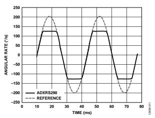
Figure 11. Rate Output Saturation Behavior
