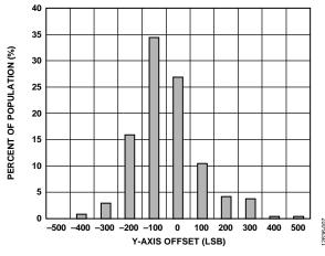
Figure 7. Y-Axis Offset at 25°C
