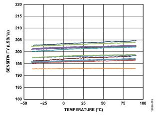
Figure 13. Y-Axis Sensitivity vs. Temperature (N = 16)
