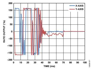
Figure 16. Start-Up Time (Standby to Measurement Mode)
