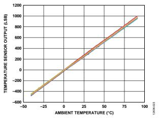
Figure 17. Temperature Sensor Output vs. Ambient Temperature (N = 16)
