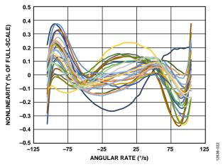
Figure 20. Rate Output Nonlinearity (N = 15)
