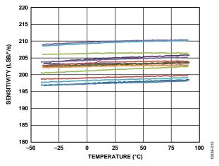
Figure 10. X-Axis Sensitivity vs. Temperature (N = 16)
