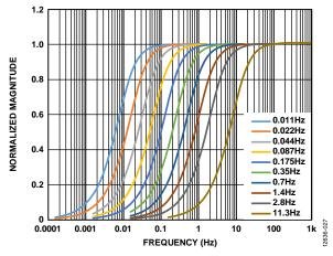
Figure 25. High-Pass Filter Frequency Response
