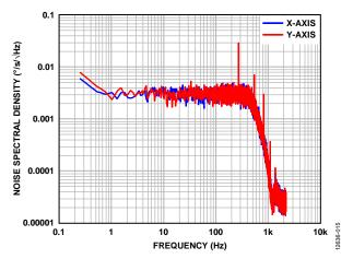
Figure 15. Typical Noise Spectral Density
