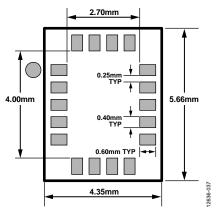
Figure 35. PCB Footprint Pattern and Dimensions
