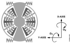
Figure 23. Simplified Gyroscope Sensing Structure
