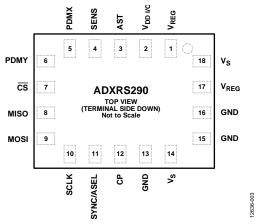
Figure 3. Pin Configuration (Top View)
