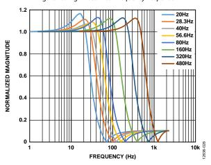
Figure 26. Low-Pass Filter Frequency Response
