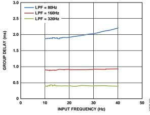
Figure 18. Low-Pass Filter Group Delay
