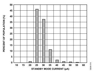
Figure 21. Standby Mode Current Consumption
