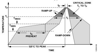
Figure 34. Recommended Soldering Profile
