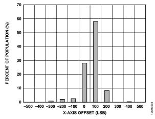
Figure 4. X-Axis Offset at 25°C
