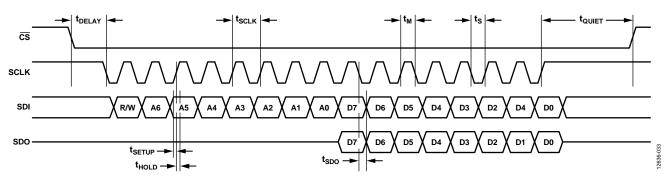
Figure 31. SPI Timing Diagram
