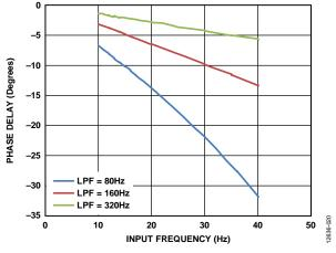
Figure 19. Low-Pass Filter Phase Delay
