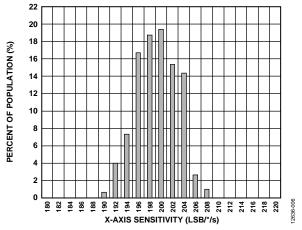
Figure 6. X-Axis Sensitivity at 25°C
