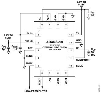
Figure 27. Recommended Application Circuit for Analog Mode Operation
