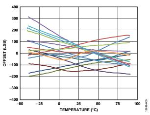
Figure 5. X-Axis Offset vs. Temperature (N = 16)
