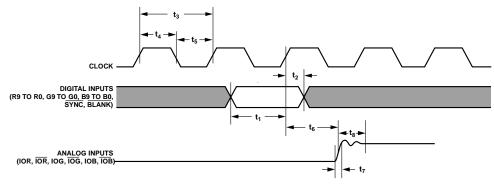
NOTES 1. OUTPUT DELAY ( $t_6$ ) MEASURED FROM THE 50% POINT OF THE RISING EDGE OF CLOCK TO THE 50% POINT OF FULL-SCALE TRANSITION. 2. OUTPUT RISE/FALL TIME ( $t_7$ ) MEASURED BETWEEN THE 10% AND 90% POINTS OF FULL-SCALE TRANSITION. 3. TRANSITION TIME ( $t_8$ ) MEASURED FROM THE 50% POINT OF FULL-SCALE TRANSITION TO WITHIN 2% OF THE FINAL OUTPUT VALUE.
