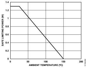
Figure 2. Thermal Derating Curve
