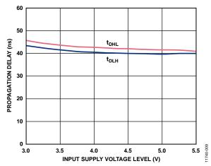
Figure 9. Typical Propagation Delay vs. Input Supply Voltage,  $V_{DDA}/V_{DDB} = 12 \text{ V}$
