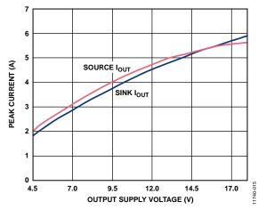
Figure 15. Typical Peak Output Current vs. Output Supply Voltage, 1.2  $\Omega$  Series Resistance
