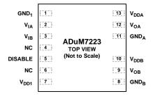
NC = NO CONNECT. NOT INTERNALLY CONNECTED.
