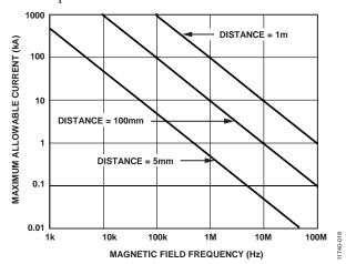
Figure 19. Maximum Allowable Current for Various Current to ADuM7223 Spacings
