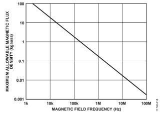
Figure 18. Maximum Allowable External Magnetic Flux Density
