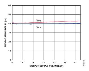
Figure 10. Typical Propagation Delay vs. Output Supply Voltage,  $V_{DD1} = 5 \text{ V}$
