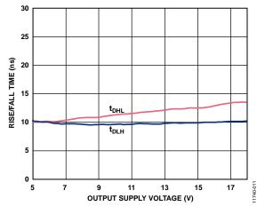
Figure 11. Typical Rise/Fall Time vs. Output Supply Voltage
