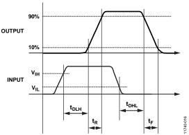
Figure 16. Propagation Delay Parameters
