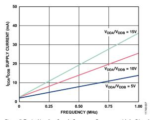
Figure 7. Typical  $I_{DDA}/I_{DDB}$  Supply Current vs. Frequency with 2 nF Load
