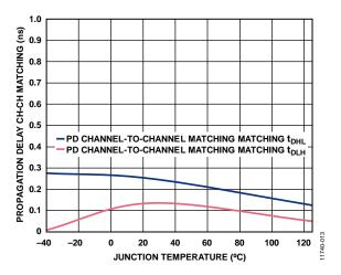
Figure 13. Typical Propagation Delay (PD) Channel-to-Channel Matching vs.  $Temperature, V_{DDA}/V_{DDB} = 12 V$
