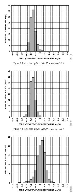
Figure 8. Z-Axis Zero-g Bias Drift,  $V_S = V_{DD I/O} = 3.3 V$
