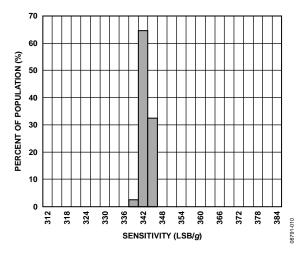
Figure 10. Y-Axis Sensitivity,  $V_S = V_{DD VO} = 3.3 V, 25^{\circ}C$
