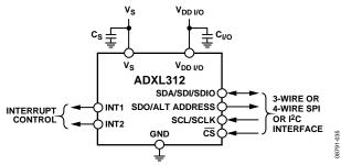
Figure 31. Application Diagram
