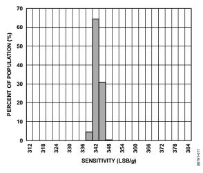
Figure 11. Z-Axis Sensitivity,  $V_S = V_{DD I/O} = 3.3 V, 25^{\circ}C$
