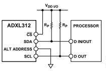
Figure 27. I<sup>2</sup>C Connection Diagram (Address 0x53)
