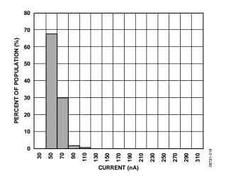
Figure 18. Standby Mode Current Consumption,  $V_S = V_{DD VO} = 3.3 V, 25^{\circ}C$
