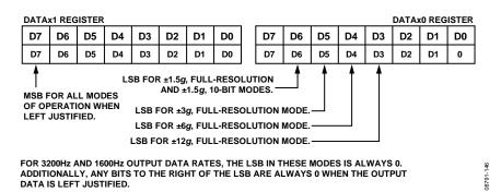
Figure 34. Data Formatting of Full-Resolution and  $\pm$ 1.5 q, 10-Bit Modes of Operation When Output Data Is Left Justified
