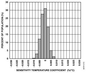
Figure 13. Y-Axis Sensitivity Temperature Coefficient,  $V_S = V_{DD I/O} = 3.3 V$
