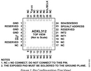
Figure 2. Pin Configuration (Top View)
