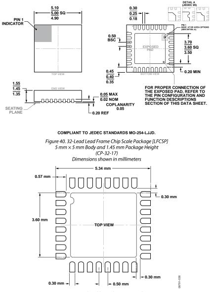
Figure 41. Sample Solder Pad Layout (Land Pattern)
