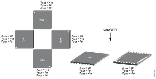
Figure 38. Output Response vs. Orientation to Gravity
