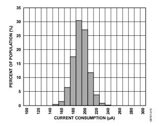
Figure 19. Current Consumption, Measurement Mode, Data Rate = 100 Hz,  $V_S = V_{DD \ VO} = 3.3 \ V, 25 \ ^{\circ}C$
