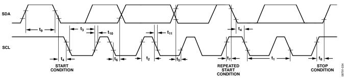
Figure 29. I<sup>2</sup>C Timing Diagram
