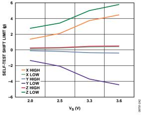
Figure 30. Self-Test Output Change Limits vs. Supply Voltage
