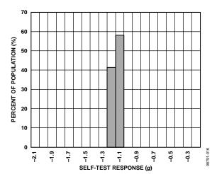
Figure 16. Y-Axis Self-Test Delta, V<sub>S</sub> = V<sub>DD I/O</sub> = 3.3 V, 25°C
