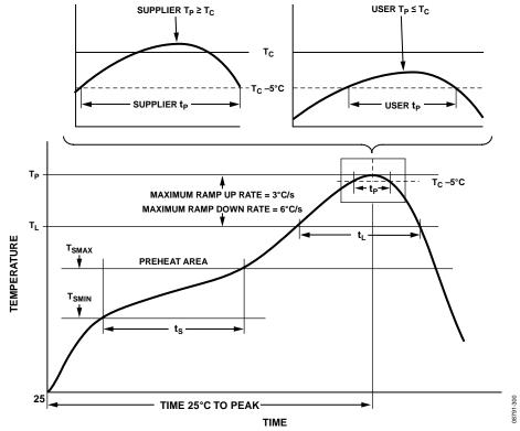
Figure 39: Recommended Soldering Profile
