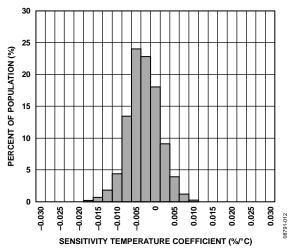
Figure 12. X-Axis Sensitivity Temperature Coefficient,  $V_S = V_{DD I/O} = 3.3 V$
