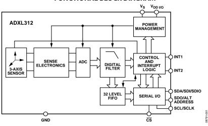
Figure 1. ADXL312 Simplified Block Diagram
