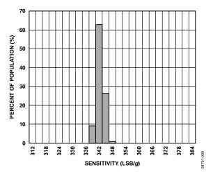
Figure 9. X-Axis Sensitivity,  $V_S = V_{DD I/O} = 3.3 V, 25^{\circ}C$
