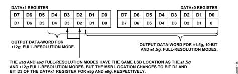
Figure 33. Data Formatting of Full-Resolution and  $\pm$ 1.5 g, 10-Bit Modes of Operation When Output Data Is Right Justified
