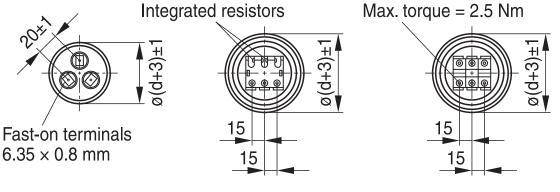
Creepage distance > 12.7 mm Distance in air > 10 mm
