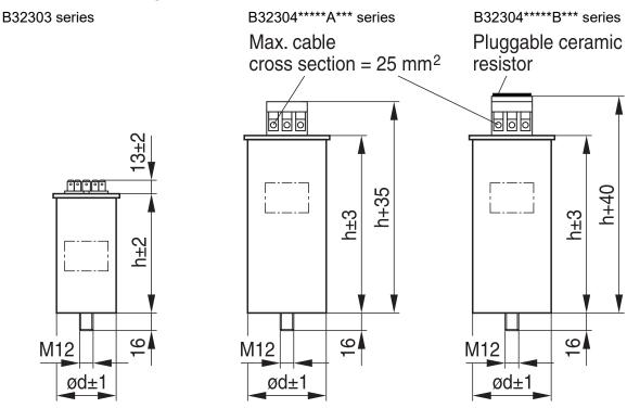
Torque = 10 Nm, Toothed washer J12 DIN 6797, Hex nut BM 12 DIN 439
