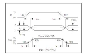
Fig 3 Driver Propagation Delays
