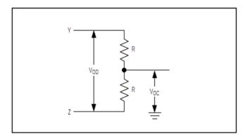
Fig 1 Driver DC Test Load
