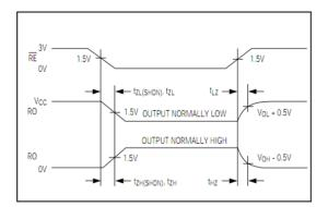
Fig 9 Receiver Enable and Disable Times
