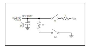
Fig 8 Receiver Enable/Disable Timing Test Load
