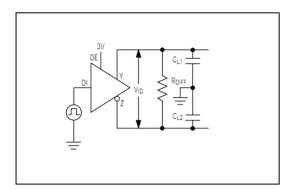
Fig 2 Driver Timing Test Circuit
