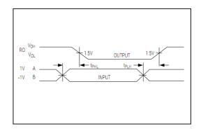
Fig 7 Receiver Propagation Delays
