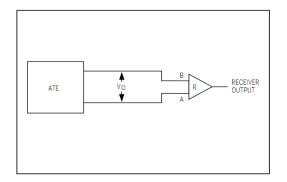
Fig 6 Receiver Propagation Delay Test Circuit
