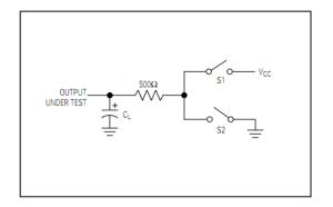
Fig 4 Driver Enable/Disable Timing Test Load
