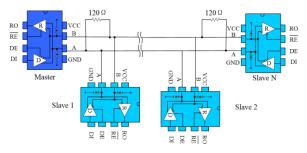
Fig 10 Backbone cable type RS485 communications network
