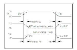
Fig 5 Driver Enable and Disable Times
