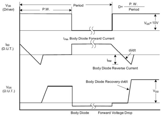
Fig. 1.2 Peak Diode Recovery dv/dt Waveforms
