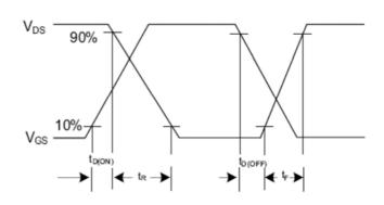
Fig. 2.2 Switching Waveforms
