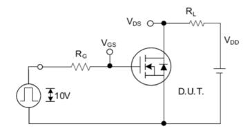
Fig. 2.1 Switching Test Circuit
