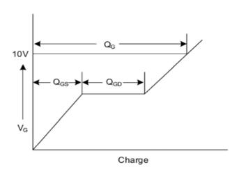
Fig. 3.2 Gate Charge Waveform
