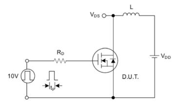
Fig. 4.1 Unclamped Inductive Switching Test Circuit
