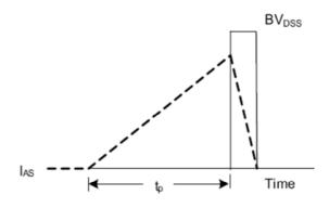
Fig. 4.2 Unclamped Inductive Switching Waveforms
