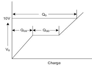
Fig. 3.2 Gate Charge Waveform
