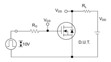
Fig. 2.1 Switching Test Circuit
