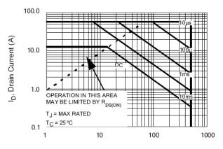
V<sub>DS</sub>, Drain-to-Source Voltage (V)
