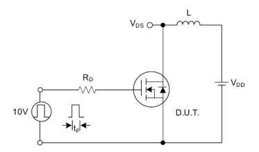
Fig. 4.1 Unclamped Inductive Switching Test Circuit
