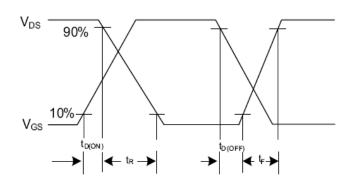
Fig. 2.2 Switching Waveforms
