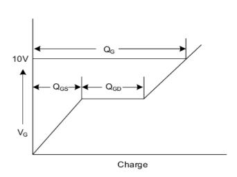
Fig. 3.2 Gate Charge Waveform
