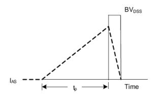
Fig. 4.2 Unclamped Inductive Switching Waveforms
