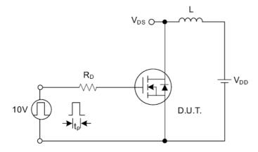
Fig. 4.1 Unclamped Inductive Switching Test Circuit
