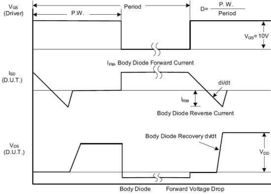
Fig. 1.2 Peak Diode Recovery dv/dt Waveforms
