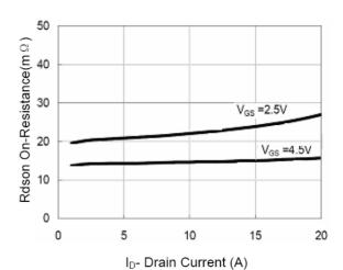
Figure 4 Drain-Source On-Resistance
