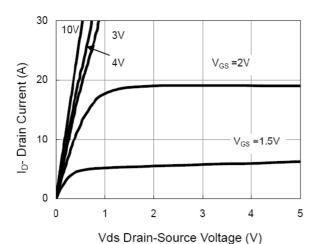
Figure 3 Output Characteristics
