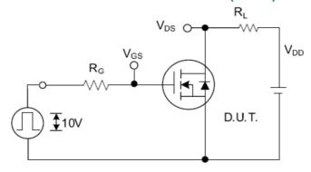
Fig. 2.1 Switching Test Circuit
