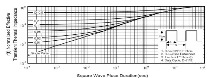
Figure 12 Normalized Maximum Transient Thermal Impedance
