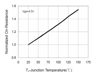
Figure 6 Drain-Source On-Resistance
