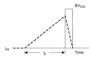
Fig. 4.2 Unclamped Inductive Switching Waveforms
