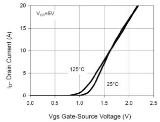
Figure 5 Transfer Characteristics
