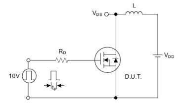
Fig. 4.1 Unclamped Inductive Switching Test Circuit
