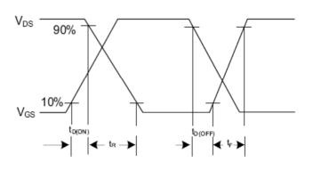
Fig. 2.2 Switching Waveforms
