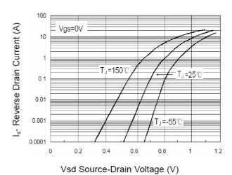
Figure 10 Source- Drain Diode Forward
