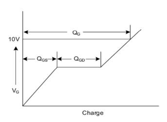
Fig. 3.2 Gate Charge Waveform
