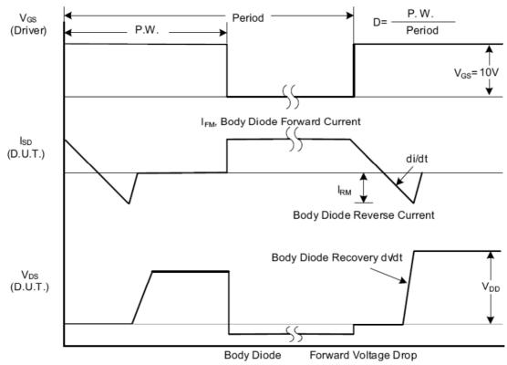
Fig. 1.2 Peak Diode Recovery dv/dt Waveforms
