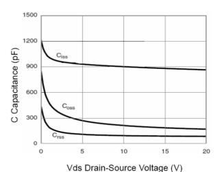
Figure 8 Capacitance vs Vds
