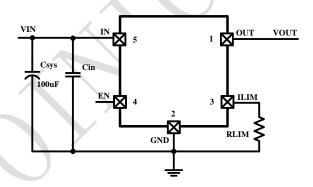
Figure 1 IP2680 Typical Application Circuit
