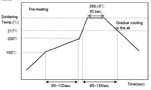
[Reflow Soldering Conditions]
