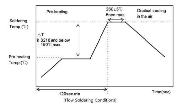
Take caution not to exceed peak temperature (260°C) and time (5sec) as shown. In case of flow soldering, only 1608(0603inch), 2012(0805inch), 3216(1206inch) case size are recommended to use.
