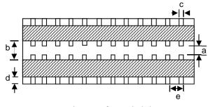
(Substrate for bending strength test)
