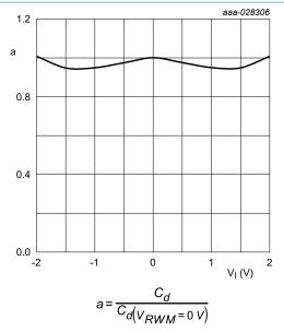
Fig. 4. Relative capacitance as a function of input voltage; typical values
