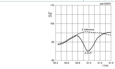
Fig. 5. Differential Time Domain Reflectometer (TDR) plot; typical values
