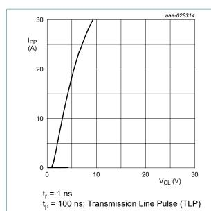
Fig. 12. Dynamic resistance with positive clamping; typical values
