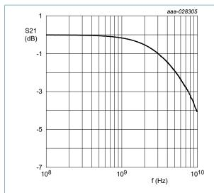
Fig. 3. Insertion loss; typical values
