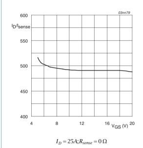
Fig 15. Drain-sense current ratio as a function of gate-source voltage; typical values
