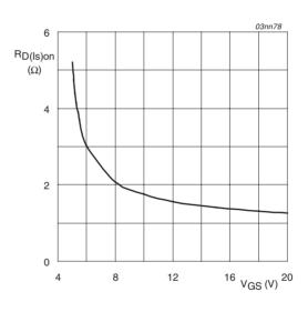
Fig 16. Drain-sense current on-state resistance as a function of gate-source voltage; typical values
