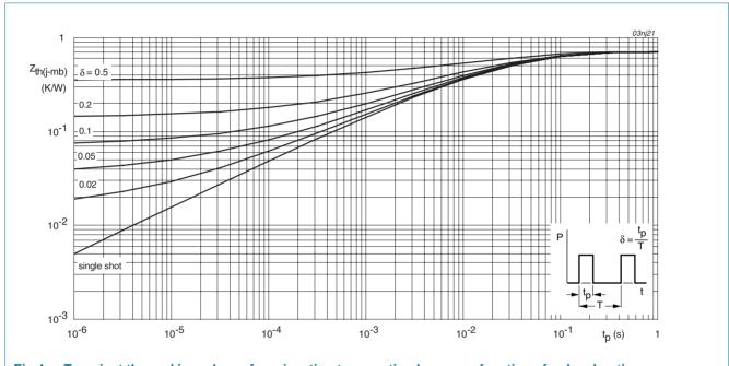
Fig 4. Transient thermal impedance from junction to mounting base as a function of pulse duration
