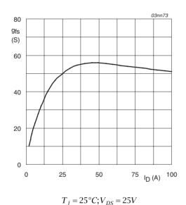
Fig 11. Forward transconductance as a function of drain current; typical values
