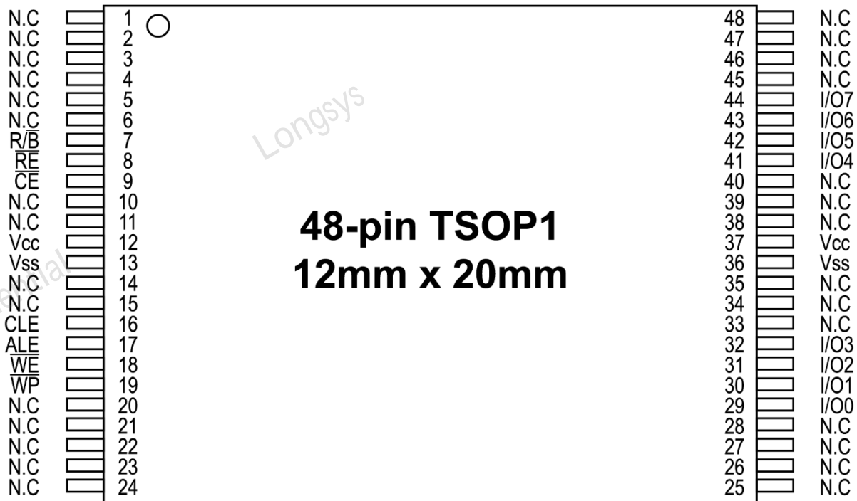
Figure 1 48-Pin TSOP1 Contact x8 Device
