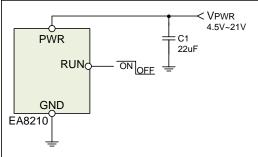
Figure 3. Enable control by RUN pin voltage
