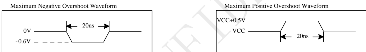
Figure 5-1 Maximum Overshoot Waveform
