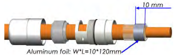
Step 4: Wrap foil over braided shielding
