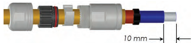
Step 6: Slide plug onto crimped terminal assembly
