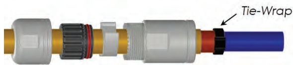
Step 3: Cut tie wrap to remove excessive material. Trim shielding flush to edge of tie wrap
