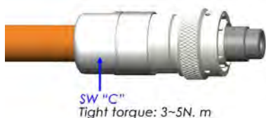
Step 9: Attach and tighten backshell as shown
