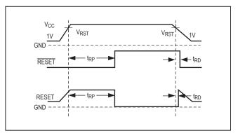
Figure 2. Reset Timing Diagram
