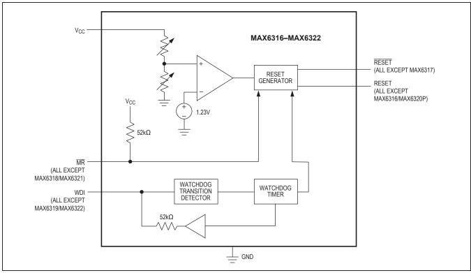
Figure 1. Functional Diagram
