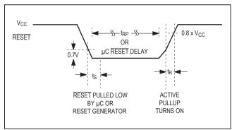
Figure 5. Bidirectional RESET Timing Diagram
