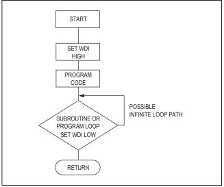
Figure 10. Watchdog Flow Diagram
