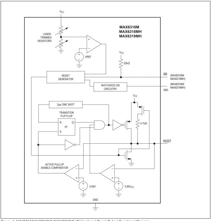
Figure 4. MAX6316/MAX6318MH/MAX6319MH Bidirectional Reset Output Functional Diagram
