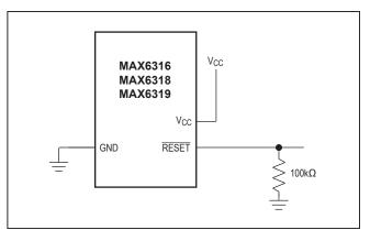
Figure 8. Ensuring  $\overrightarrow{RESET}$  Valid to  $V_{CC} = 0V$  on Active-Low Push/Pull and Bidirectional Outputs
