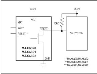
Figure 6. MAX6320P/MAX6321HP/MAX6322HP Open-Drain RESET Output Allows Use with Multiple Supplies
