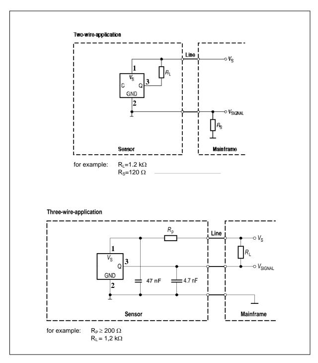
Figure 2: Application Circuits (capacitors to be added externally)
