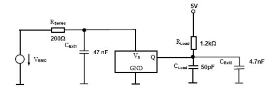
Figure 3: Test Circuit for EMC tests
