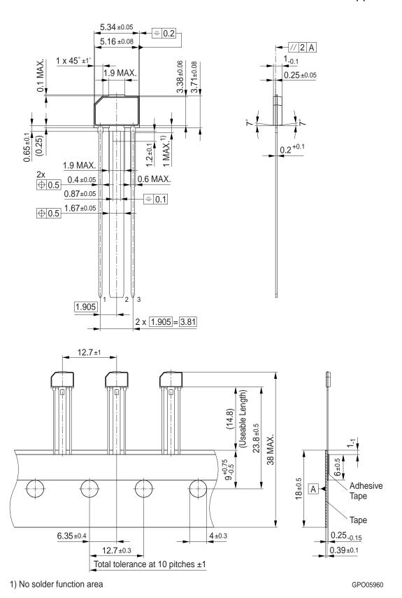
Figure 4: PG-SSO-3-6 package drawing
