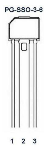
Figure 1: Pin configuration in PG-SSO-3-6
