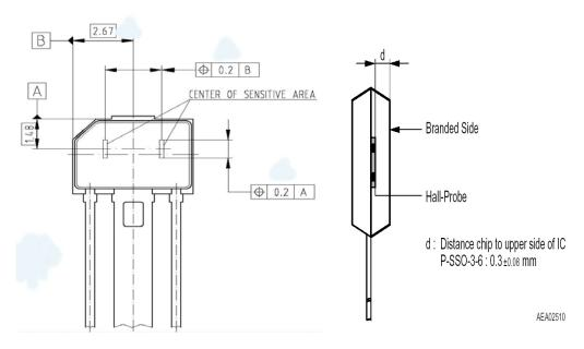
Figure 5: Hall probe spacing in the PG-SSO-3-6 package
